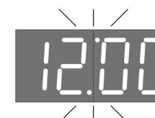
\* To change the program cycle from daily to weekly week and vice versa ,in the time setting mode (see p. ③), simultaneously press and hold both buttons, then no later than in 1.5 seconds take out and reinsert the plug into the socket and only after the appearance of the corresponding indication release the button.
