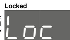
↙ **Buttons lock (child lock, etc.).** Turn on the heater to the mains while holding down the '+' button and hold it until the appropriate indication and audible confirmation appears. After this the heater will react only with a low beep when buttons are pressed.
